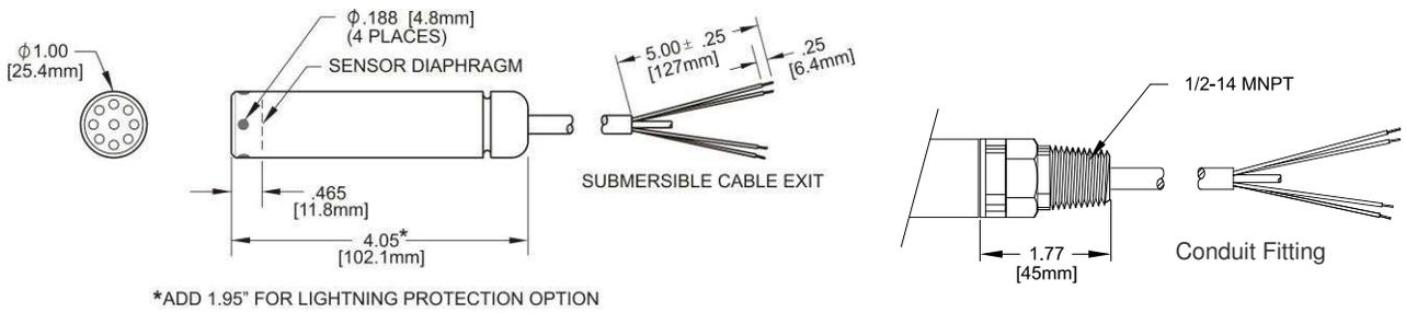
Gland Cable Seal Configuration for ETFE Cable
