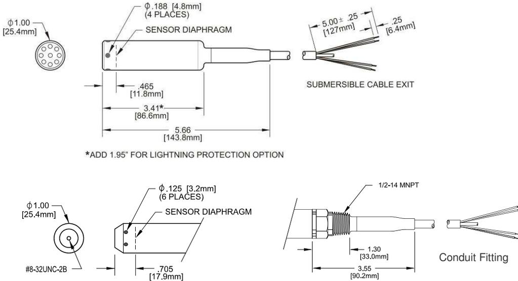
Molded Cable Seal Configuration for Polyurethane Cable
