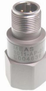
The Model 8011 & 8012 are internally shielded rugged 4-20mA accelerometers. The accelerometers are available in ranges from  $\pm 5g$  to  $\pm 50g$ , in either RMS or Peak acceleration output options. The model 8011 features a top exit MIL-C-5015 connector while the model 8012 features an integral cable. The units are hermetically sealed and are designed for operating in temperature ranges from -40°C to +85°C.
