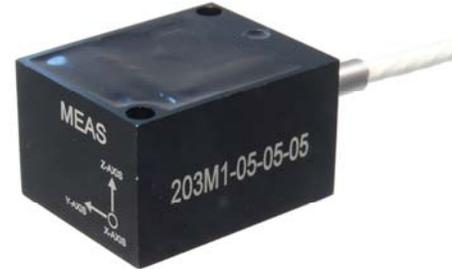
The **Model 203** is a low noise triaxial accelerometer offering both static and dynamic response. The accelerometer is packaged in an anodized aluminum housing with an integral cable. It is offered in ranges from  $\pm 2g$  to  $\pm 100g$ . Featuring gas damped MEMS sensing elements, the model 203 provides a flat frequency response to 100Hz over an operating temperature range of  $-40^{\circ}\text{C}$  to  $+125^{\circ}\text{C}$ .
