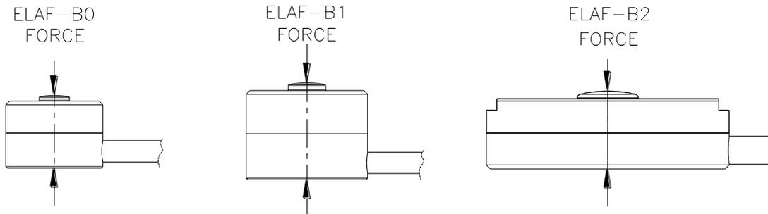
BO, B1 & B2: SPHERICAL CONTACT ON THE TOP AND FLAT SURFACE ON THE BOTTOM
