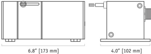
The PT5MA potentiometric cable-extension transducer uses a unique thermoplastic cable that has virtually an infinite fatigue life. This cable, known as V62, has properties that are superior for high cycle and rugged applications.
