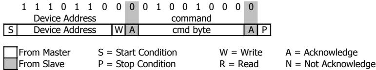
Figure 8: I<sup>2</sup>C command to initiate a pressure conversion (OSR=4096, typ=D1)
