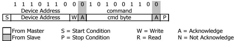
Figure 6: I<sup>2</sup>C Command to read memory address= 011
