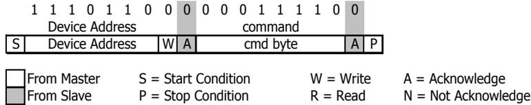
Figure 5: I<sup>2</sup>C Reset Command
