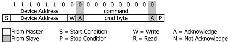
Figure 9: I<sup>2</sup>C ADC read sequence
