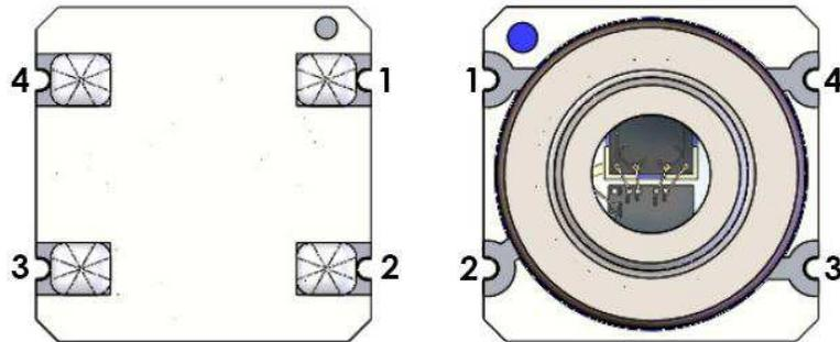
Figure 13: pin configuration
