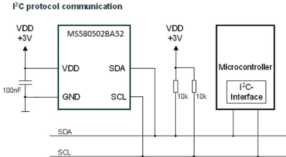
Figure 12: Typical application circuit with I<sup>2</sup>C protocol communication
