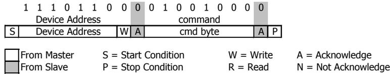
I<sup>2</sup>C command to initiate a pressure conversion (OSR=4096, typ=D1)
