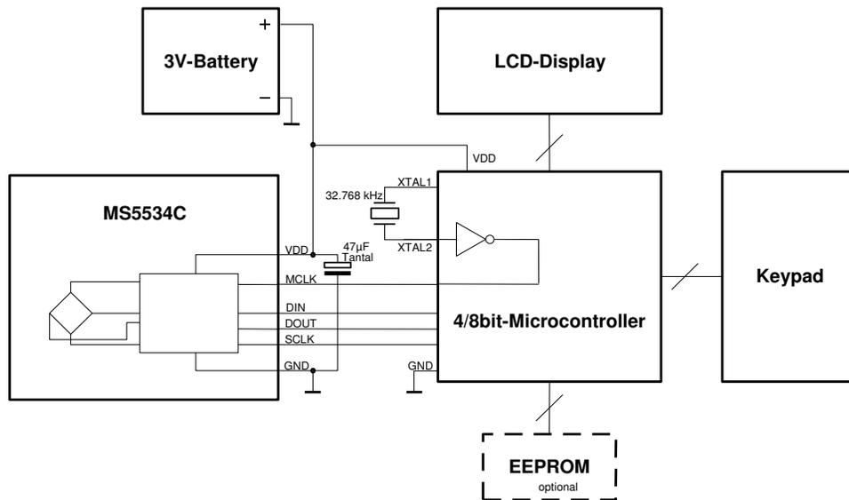
Figure 7: Demonstration of MS5534C in a mobile altimeter
