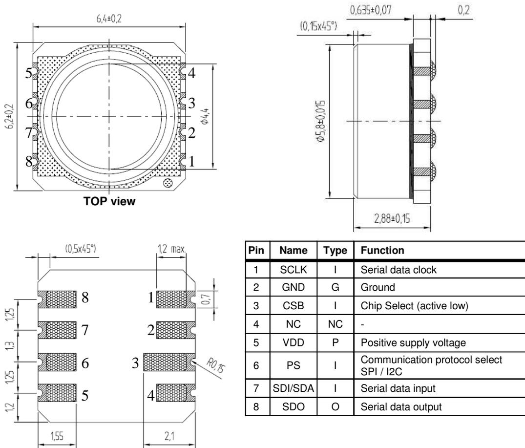
Figure 18: MS5803-01BA package outlines, pin configuration and description
