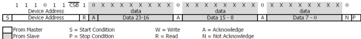
Figure 6: I<sup>2</sup>C pressure response (D1) on 24 bit from MS5803-01BA
