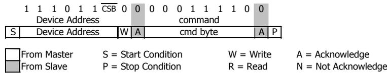
Figure 3: I<sup>2</sup>C Reset Command
