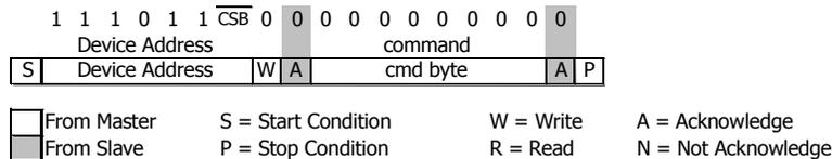
Figure 5: I<sup>2</sup>C ADC read sequence
